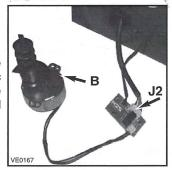
12 Mount the new damper actuator assembly to the unit. Plug the unit and turn it on.
