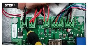
4. After the test is completed, unplug the unit and replace the black wire from the cord in its original position identified "Line".
