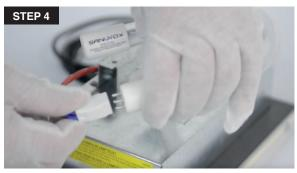
4. While holding the porcelain end-cap (with 4 pins), carefully push the white connector onto the four pins. The plug is designed so that it can only be installed one way. You may have to rotate the socket 90° to line up the pins with the holes. The connector will fit into position.
