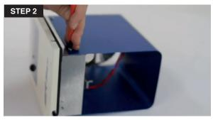
2. Release the reflecting tube by removing the 2 screws on each side to access the lamp.
