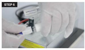
6. While holding the porcelain end-cap (with 4 pins), carefully push the white connector onto the four pins. The plug is designed so that it can only be installed one way. You may have to rotate the socket 90° to line up the pins with the holes. The connector will fit into position.
