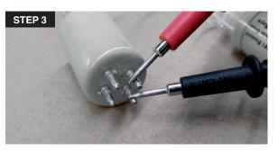
3. Using an ohmmeter place 1 probe on 1 of the 4 pins and by sensing the 3 remaining pins, one should have continuity. Make sure the 2 remaining pins also have continuity. When both sets of pins test good for continuity, it can be assumed that the lamp is good.
