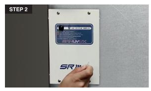
2. Use a small object similar to a paper clip and insert it into the reset hole in order to be able to press the reset button.
