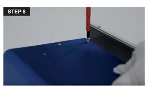
8. Once the UV lamp is installed, reinstall the reflecting tube. It is important to note that the air should first flow through the turbulator before moving in front of the UV lamp.
