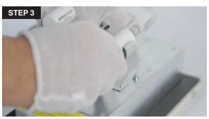
3. Remove the old UV lamp from the lamp socket by opening the retaining clamp and pulling the UV lamp out.
