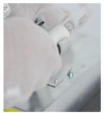
Release the reflecting tube by removing the 2 screws on each side to access the lamp. Then remove the UV lamp from the lamp socket by opening the retaining clamp and pulling the UV lamp out of the reflector chamber.
