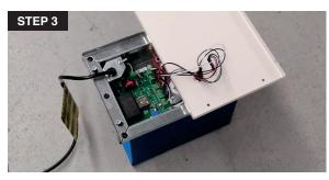
3. Place the unit down and make sure you have no direct line of sight with the lamp. Plug the power cord.
