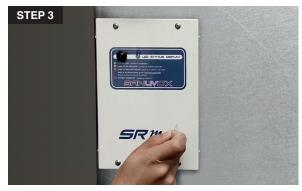
3. Press and hold the reset button for a minimum of 3 seconds. When releasing the reset button, the counter will be reset to 1096 days.
