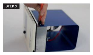
3. To install the UV lamp, release the reflecting tube by removing the 2 screws on each side.
