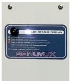
3. First turn ON the power switch and then, press the reset button. You have 5 seconds from the moment the unit is powered to press the reset button to activate the airflow detection. Every time you press the button you will notice that the LED color will either be "Blue" or "White". Once the LED is "Blue", wait 5 seconds while holding the reset button for the control circuit to save the setting.
