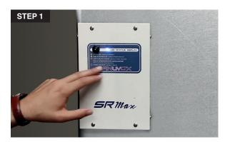
1. To reset the lamp timer the unit needs to be powered and turned ON. The status LED should either be "Green" or "Blue" (heartbeat).
