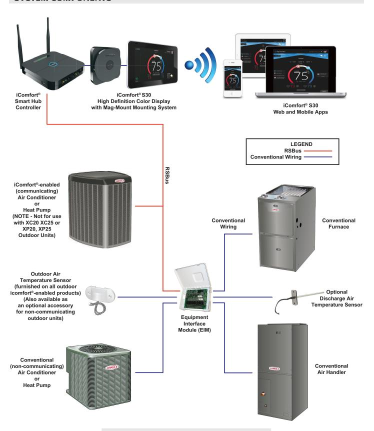
ATTENTION - The Lennox iComfort® Thermostat with Equipment Interface Module (EIM) will work with most 24VAC furnaces, air conditioners, air handlers and heat pumps (up to 3 stages of heat and 2 stages of cooling), EXCEPT it will NOT work with any brand of communicating HVAC equipment other than LENNOX®.
