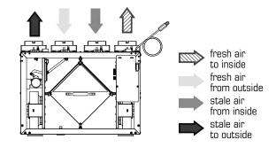
Clearance of 17" (432 mm) in front of the unit is recommended for removal of core. All units feature three foot plug-in power cord with 3-prong plug.
